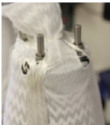
Example of split tape to veer around braid/features
